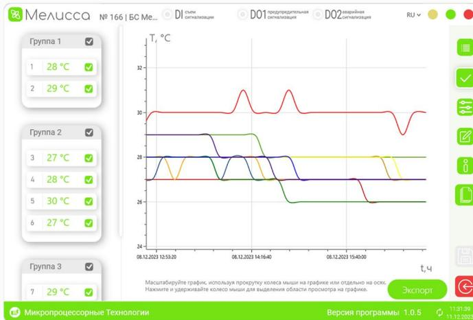
The screenshot shows a temperature history graph for six sensors. The y-axis represents temperature in °C (24 to 32), and the x-axis represents time (08.12.2023 12:33:20 to 15:40:00). The graph shows temperature fluctuations for each sensor over time.
